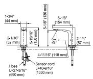
■Mounting deck thickness: 1/4" (5 mm) - 2" (50 mm) ■Spout hole: Ø1-1/4" (Ø32 mm) - Ø1-3/8" (Ø35 mm)
